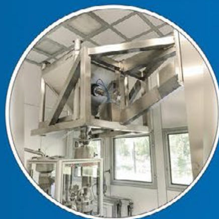
Lifting Column for Bin with an integrated vibration system
