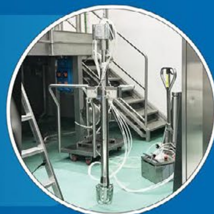
Lump Breaker Lance with spring balancer
