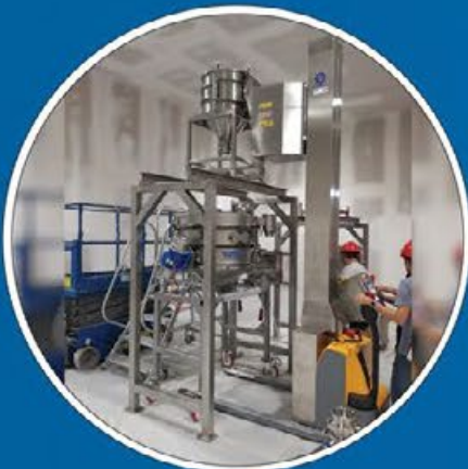
Motorized Lifting Column for Drums Discharge through Sieve
