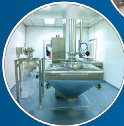
Bin Blending Column for Mill loading
