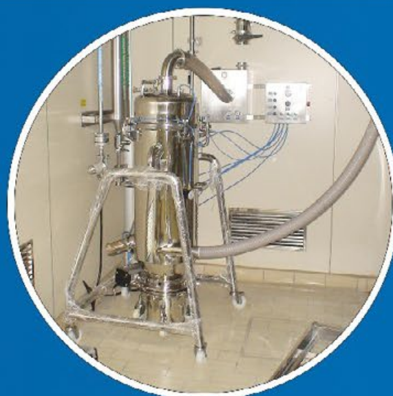
Filtervac FT400 for Bicone loading
