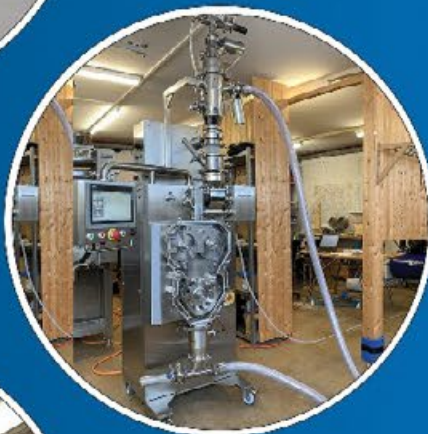
Vacuum Conveyor to load a Roller Compactor
