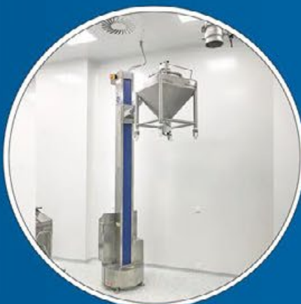
Stationary Bin Lifter with brushless motor for the correct position of the Split Valve
