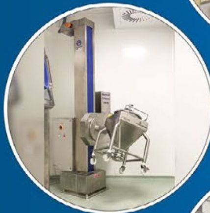
Fixed Bin Blender Column with Clamp Connection for Bin connection
