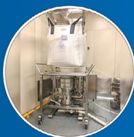
Mobile Closing System integrated with CIP
