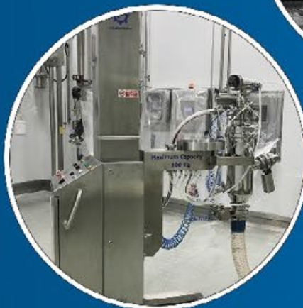
Vacuum Transfer System installed on Mobile Lifting Column
