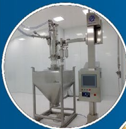
Vacuum Conveyor charging Bin from Several Big Bag unloading Structure
