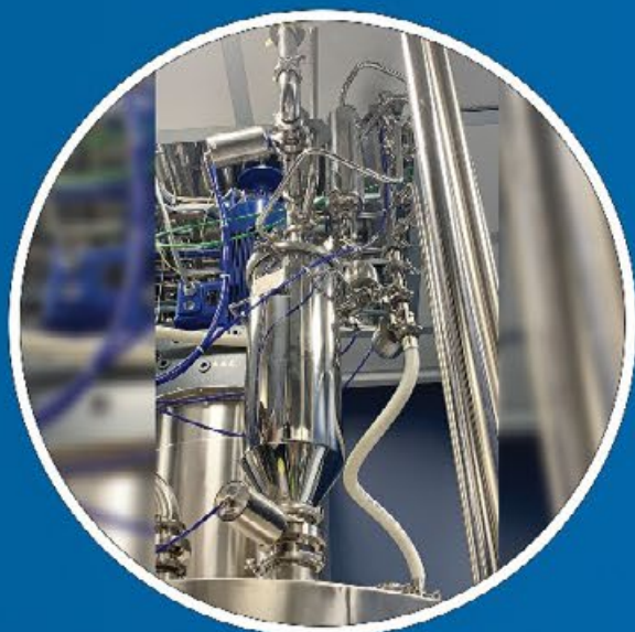
Filtervac FT200 for reactor charging
