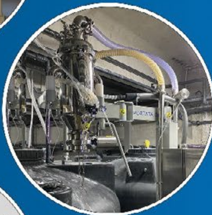
Vacuum Conveyor on a arm for charging a solis
