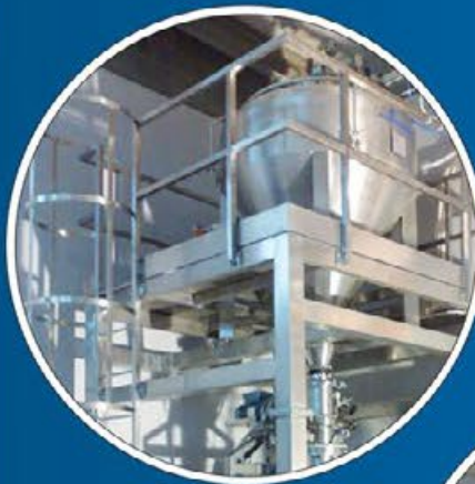
VTS Hoppervac for powder dosing system to charge a mixer
