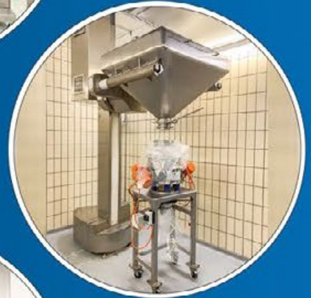
Bin Blending Column for Mill loading
