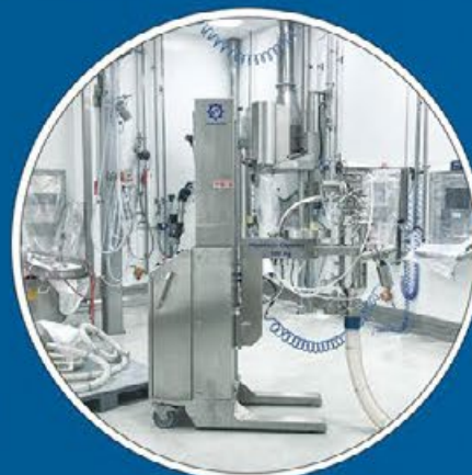
Automatic Mobile Lifting Column for Vacuum Conveyor
