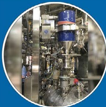
Fixed Automatic Drum Lifter for Reactor Loading
