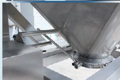
Automatic Valve Opening System
