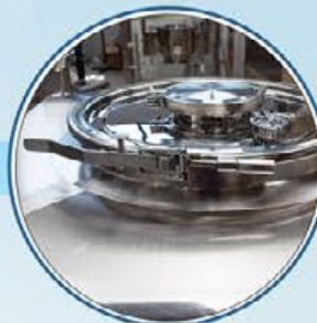
Tri-Clamp Closing for Lid with Safety Pin
