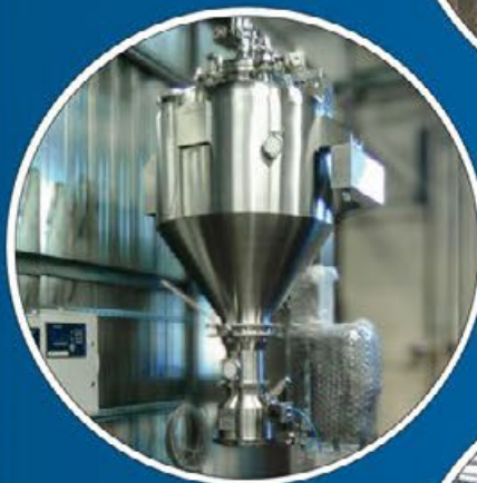
Vacuum Conveyor Hoppervac on a fixed column which discharge in drums
