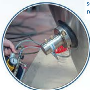
Pneumatic Vibrator with Suction Cup for easier product unloading
