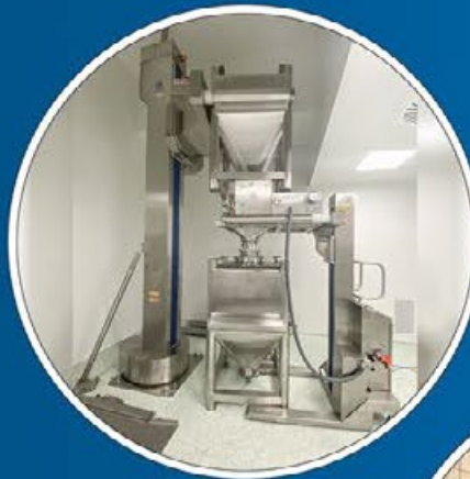
Blending and discharging System from Bin-to-Bin by Mill
