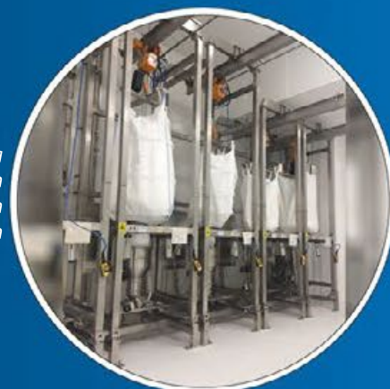
Integrated Big Bag Unloading System with Vacuum Conveyor for Bin
