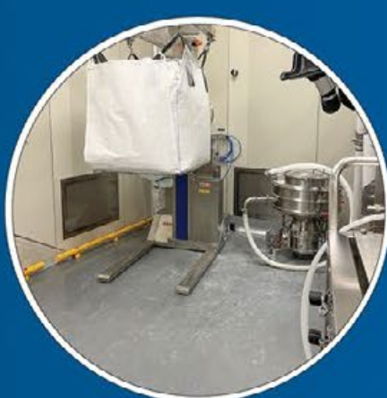
Mobile Lifting Column for Big Bag Unloading
