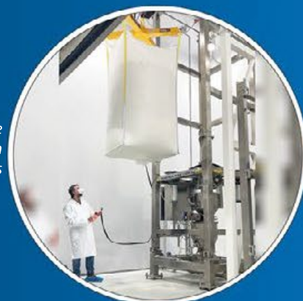
Big Bag Discharge Station installed on load cells
